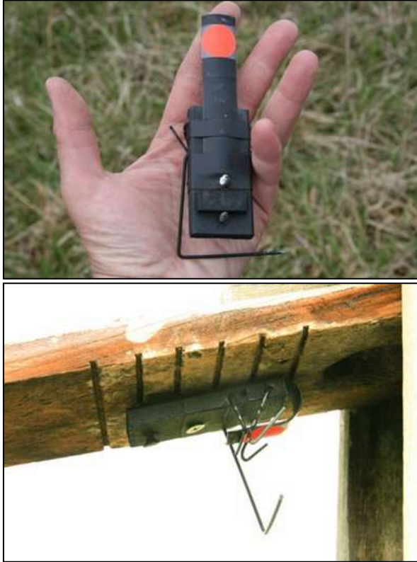
Figure 1 – (Top) Gilbertson nest-trap (bottom) Inside view of a nest box with the nest-trap set. Photos credits: http://juliezickefoose.blogspot.ca .
