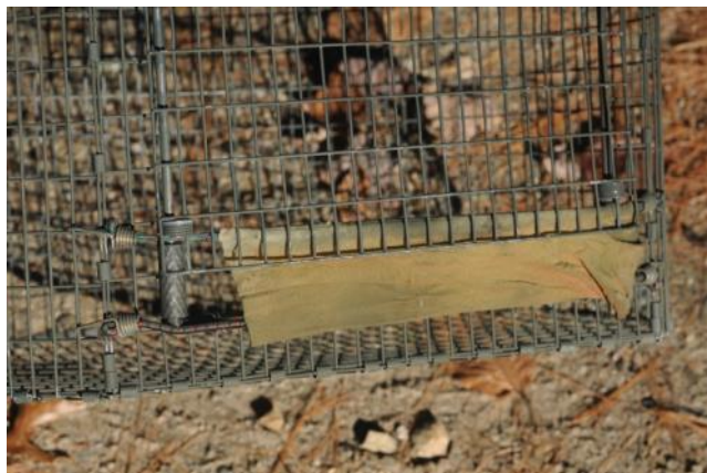
Figure 9. Detail of the “slide” style door cage trap, with added padding at bottom. Note that there is a built-in gap at the bottom of the door travel that is closed by a piece of nylon stocking stretched over 2 small bungees (photo: Anthony Hill).
