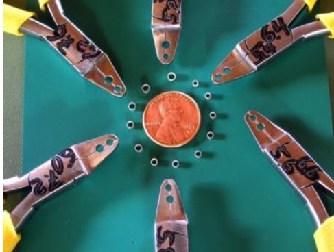
Figure 31. Pliers must match band size for correct closure (photo: Lee Rogers).
